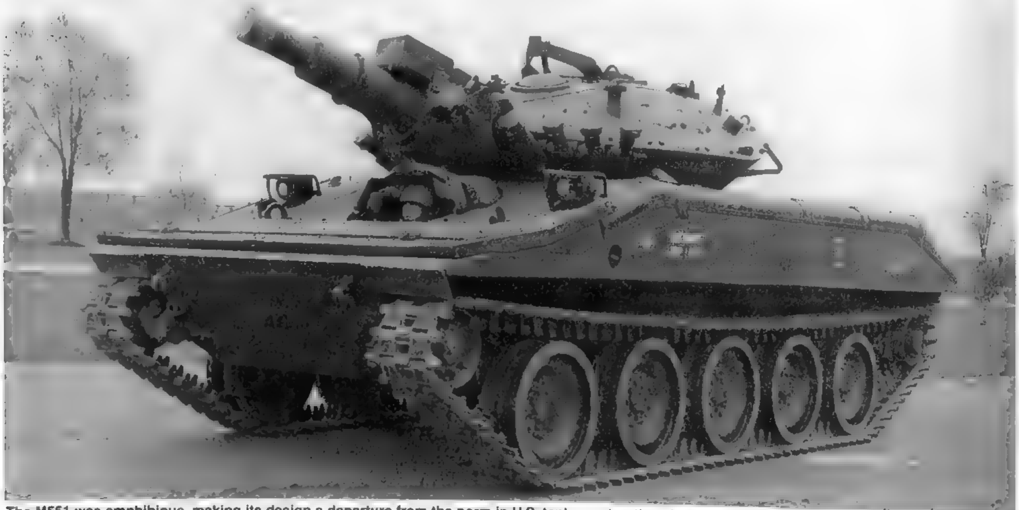
The M551 was amphibious, making its design a departure from the norm in U.S. tank construction. Across the glacis, just in front of the driver, the surf shield is folded down in its normal travel position. The rotary driver for the hatch, grenade launchers, and empty mount for the commander's machine
